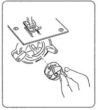
To remove bobbin case from shuttle, pull open latch of bobbin case. Pull bobbin case straight out of shuttle.
